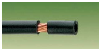
Partial stripping of the insulation
